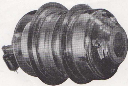
The Mullard image converter tube shown, the first of its kind which is entirely electrostatically focussed, has a built-in electron-optical zoom lens.
