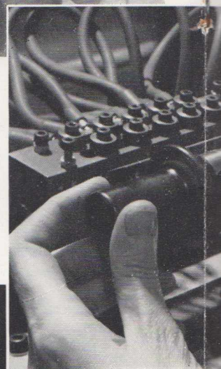
3. The major components of the gun are held together by sintered glass multi-form rods. The components are accurately positioned in a jig and their relative positions fixed immovably by their fixing lugs, which are pushed into the heated rods, as in this picture. An important point in this process is the alignment of the gas burners so as to heat the glass in the exact places required
