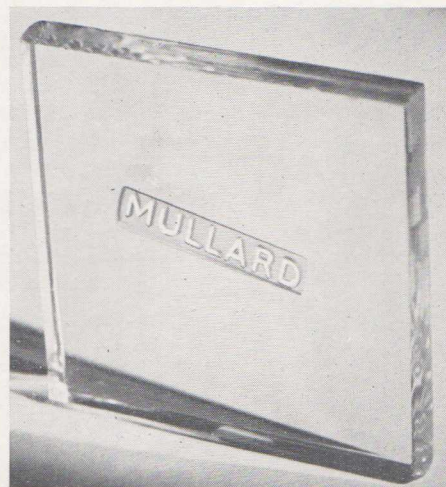
Figure 4 —A brass printing block produced this design in a single operation.
