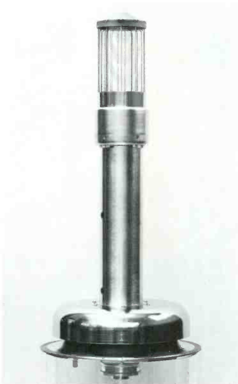
Figure 1 — Cathode-Grid and Mounting Assembly of ML-LPT17.
