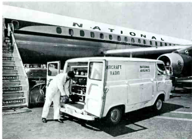
Figure 2 — The aircraft radio truck delivers a DME to a waiting DC-8. Dual DME and Transponder installations are used on these and other National aircraft.
