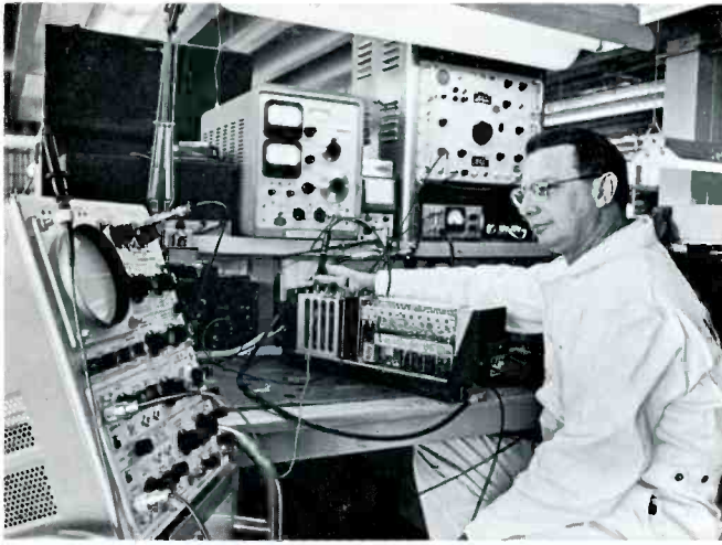
Figure 4 — The Collins 621-A transponder is adjusted in for peak performance. Cavity for the Machlett ML-7815 is visible at the left of the transponder unit.
