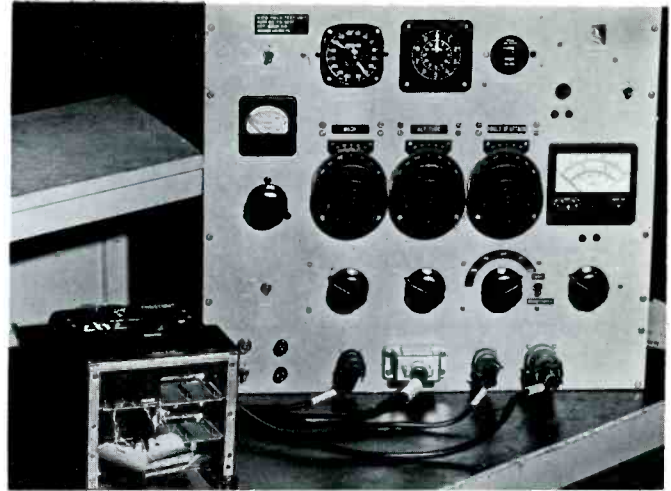
Figure 5 — KIFIS test unit, KIFIS at left, readout equipment at right. The KIFIS system provides accurate instrumentation data for the pilot.
