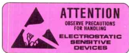
Figure 4. Approved Label for Electrostatic Sensitive Devices
