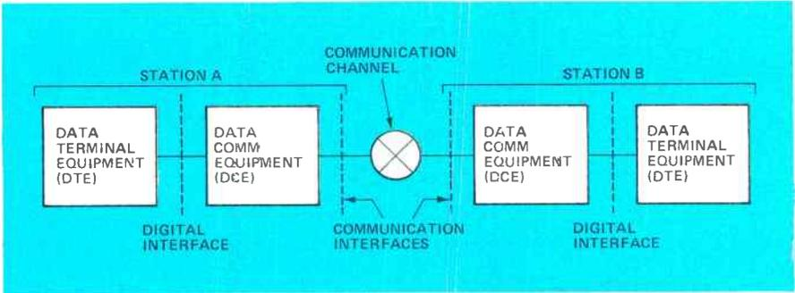
Figure 1. The data set in a data communication system ordinarily interfaces with the data terminal equipment and the communication channel.
