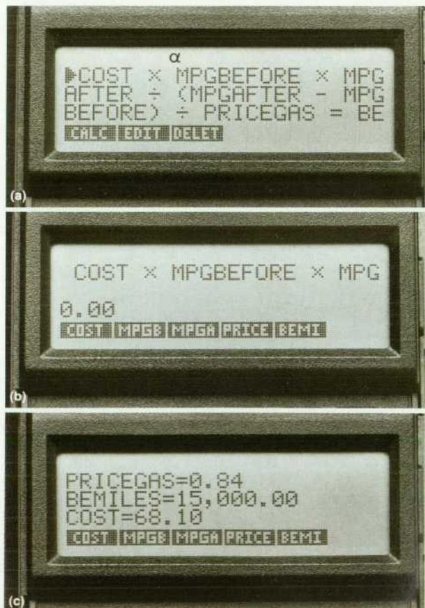
Fig. 1. Displays during solution of tune-up cost study. (a) Entry of tune-up cost equation. (b) Pressing CALC key assigns labels to softkeys as shown. (c) Break-even cost for 15,000 miles with mileage improved from 28 to 33 mpg.
