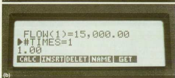
Fig. 1. HP-18C displays for cash flow analysis example. (a) Prompt display for first cash flow entry. (b) After first entry of 15,000 is input, the display prompts for the number of times entry occurs. A value of 1.00 is displayed as a default value. (c) Pressing the INPUT key prompts for the next entry. (d) After completing the cash flow entries, pressing the CALC softkey gives this display. Entering the desired interest value and pressing the 1% key then allows calculation of the net present value, net uniform series, or net future value.
