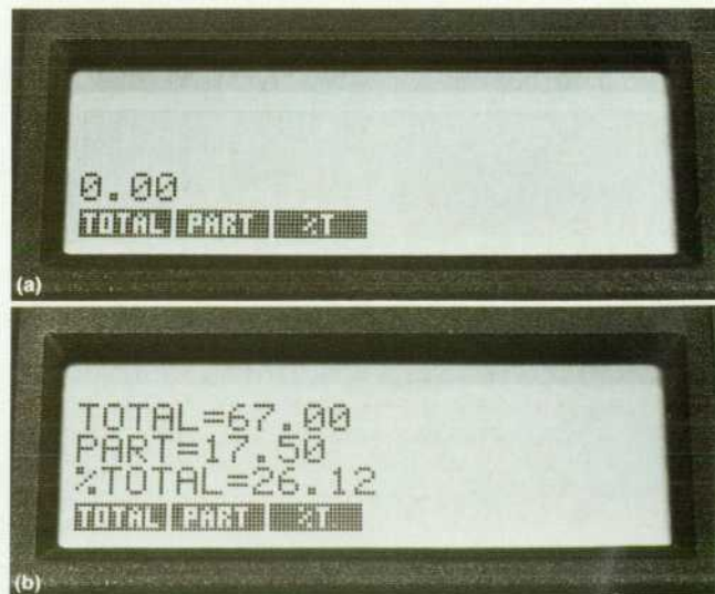
Fig. 4. Use of the HP-18C's softkey user interface. (a) %TOTL menu of BUS application. (b) Answer to determining what percentage of 67 a value of 17.5 is.
