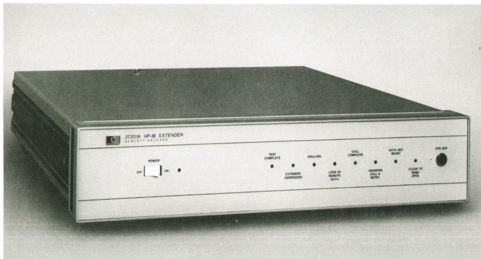
Fig. 1. The Hewlett-Packard Model 37201A HP-IB Extender converts standard HP Interface Bus activity into a serial form for communication via normal full-duplex modems or twin-pair cable. Functioning in pairs, extenders enable two distant clusters of bus-interfaced instruments to operate as one.
