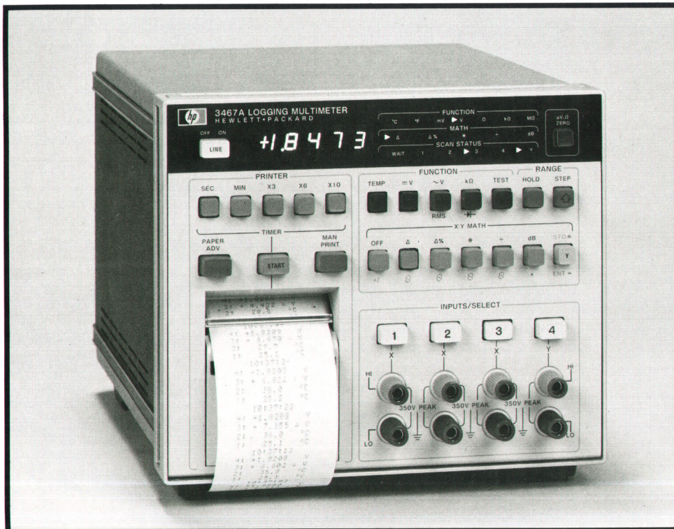
Fig. 1. The Model 3467A Logging Multimeter is basically a 4½-digit multimeter with a built-in four-channel scanner and a printer, all controlled by an internal microprocessor. The microprocessor can also translate raw measurement data into more useful forms, such as linearizing and converting thermistor measurements to give readings directly in °F or °C.
