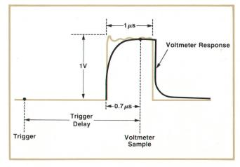
**Fig. 4.** Model 3437A Systems Voltmeter can be programmed to sample and read the amplitude of a pulse at a point in time precisely related to a trigger by the voltmeter's programmable delay. Uncertainty (jitter) in the location of the sample is less than 10 ns. The voltmeter will be accurate to at least 2% within 0.7 μs after the pulse leading edge.
