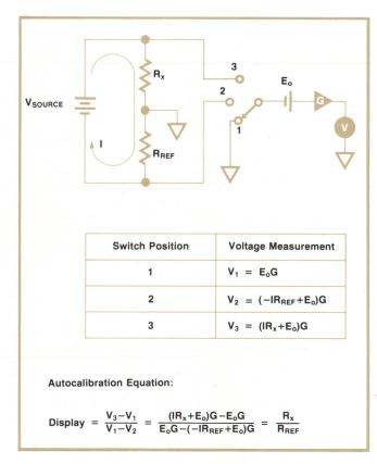
**Fig. 8.** A technique for calibrating a single range of an ohmmeter. This can be extended to three ranges by programming the amplifier to increase the gain  $10\times$  when measuring  $V_2$  or  $V_3$  (and  $V_1$  as appropriate).
