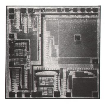
**Fig. 2.** Fine-line resistor set used in the Model 3465A Digital Multimeter is on a substrate measuring  $4.5 \times 4.5$  mm. The square area in the upper right is a  $10\text{-}M\Omega$  resistor in a square spiral pattern. With a 5-micron line width and 5-micron spacing, the lines are indistinguishable in this photo.
