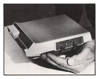
**Fig. 1.** Both inputs to the Model 3476A Digital Multimeter located on the side of the instrument, are fused. Sliding the small panel to the right aligns the input holes with the fuses, making them readily accessible for replacement.
