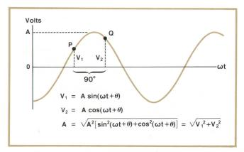
**Fig. 1.** By measuring the instantaneous level of a sine wave at two points, P and Q, 90° apart, the peak amplitude and rms values of a sine wave can be calculated. Points P and Q can occur anywhere in the waveform as long as the 90° relationship is preserved.
