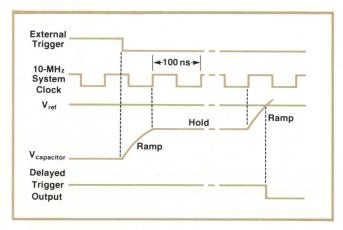
**Fig. 8.** Operation of the trigger delay interpolator. The external trigger may occur at any time with respect to a clock edge, and the delayed trigger will be generated with less than 10-ns timing uncertainty.
