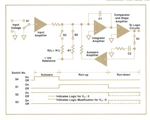
Fig. 5. Single-reference, dual slope A-to-D converter is autozeroed while switch S2 is closed. Opening S2 during integrator discharge is then equivalent to switching to a negative reference.
