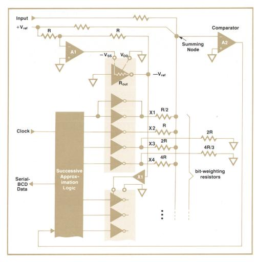
Fig. 9. Switching arrangement for part of the analog-to-digital converter. There are actually 14 bit-weighting resistors to give a 3½-digit reading in BCD format with polarity sign.
