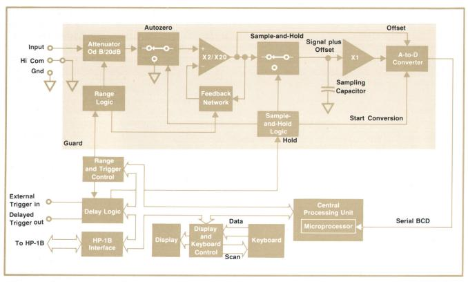
Fig. 7. Simplified block diagram of Model 3437A System Voltmeter.
