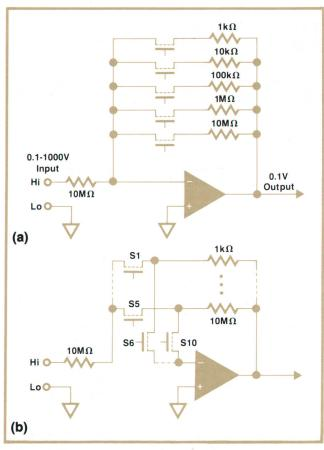
**Fig. 4.** (a) Range-switching arrangement. (b) Modification that reduces effect of MOS-transistor "on" resistance. Here, S1 and S6 are switched on to select one range, S2 and S7 (not shown) select another, and so on to S5 and S10.
