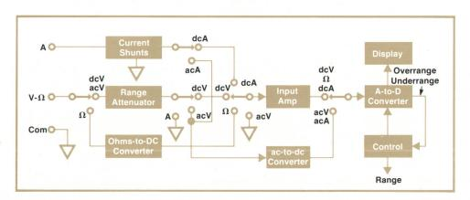
Fig. 3. Generalized block diagram of a digital multimeter. Individual instruments may differ in details.
