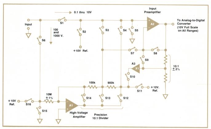
**Fig. 6.** Simplified diagram of the circuit that performs the autocalibration in the Model 3455A Digital Voltmeter. This circuit scales all inputs to the 0-10V range of the analog-to-digital converter that follows. Besides the +10V reference, the only precision components required are the two resistors in the precision divider, which are physically located in the reference module.
