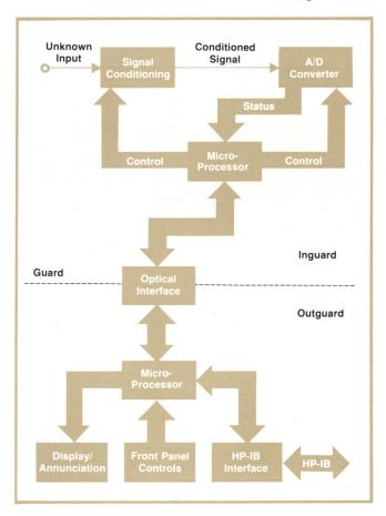
Fig. 9. Organization of Model 3455A Digital Voltmeter.
