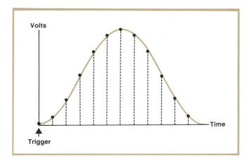
**Fig. 5.** When making measurements in bursts, Model 3437A takes several readings in response to a single trigger, 12 in this example. The time between measurements is established by the DELAY function.
