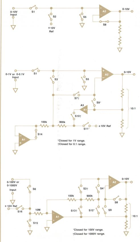
**10-volt range.** Closing switch S8 programs preamplifier A2 to a gain of 1. The unknown input, the +10-V reference, and ground are connected sequentially to the preamplifier input by switches S1, S2, and S5, just as in the basic scheme of Fig. 5.
