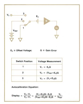
**Fig. 5.** A technique for improving the accuracy of a single-range voltmeter. The equation shows that errors caused by offset voltages and gain errors are eliminated.
