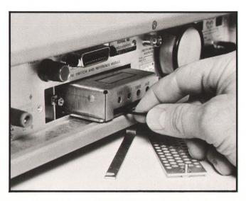
**Fig. 2.** The four adjustments that calibrate Model 3455A for do volts and ohms are in a plug-in module that can be taken to the calibration lab. Modules are interchangeable allowing an instrument to continue operating with another calibrated module plugged in.
