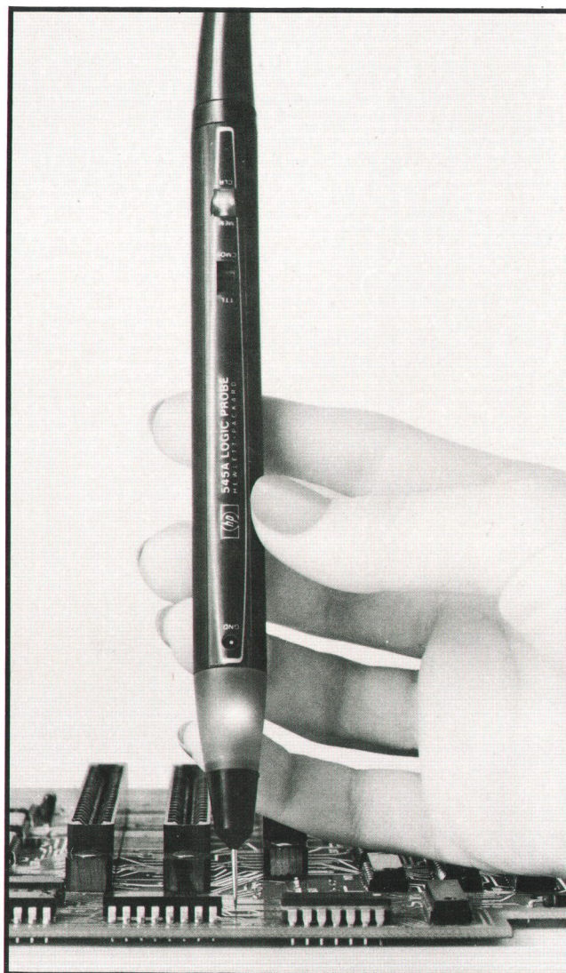
Fig. 1. Model 545A Logic Probe indicates logic levels and pulse activity at individual digital circuit nodes.
