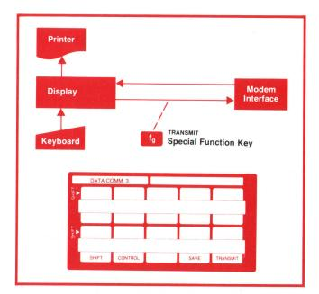
**Fig. 2.** With the Interactive ROM (Data Comm. 3) installed, received characters go directly to the calculator's display. When a carriage return character is received, the line is transferred to the printer and the display is cleared. Characters to be sent are typed into the display and sent by pressing the special function key labeled TRANSMIT. At bottom is the special function key template for the Interactive ROM.
