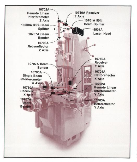
**Fig. 1.** A typical Model 5501A Laser Transducer System installed on a three-axis coordinate measuring machine. A single laser source serves all three axes. is different for different machines. However, all configurations require five choices:
