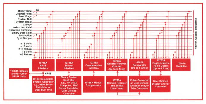
**Fig. 1.** Model 10740A Coupler serves as a housing and communications facility for the other electronic modules of the 5501A Laser Transducer System. The user selects the building blocks needed to configure a system to solve his problem.
