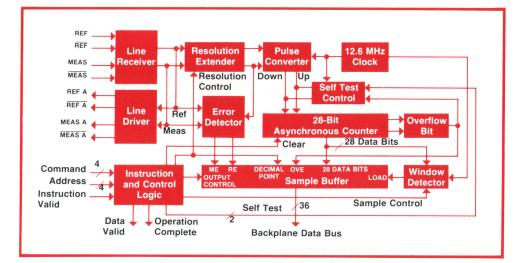
**Fig. 2.** Most systems will contain one 10760A General-Purpose Counter card for each measurement axis (up to six).
