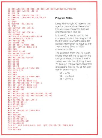
**Fig. 3.** A BASIC-language program for a 9830A Calculator used as a timesharing terminal to plot data received from an HP 2000 Timeshared Computer System.
