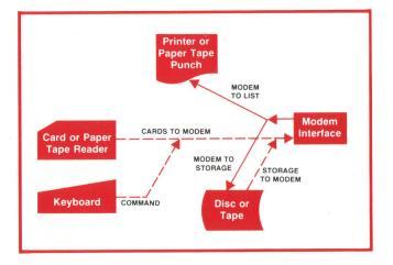
**Fig. 6.** 9830A batch terminal on-line operations. Special function keys cause information to be transferred in various ways.
