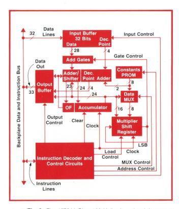
**Fig. 3.** The 10761A Binary Multiplier is optional. It converts uncompensated fringe (quarter-wave) displacement data from the 10760A Counters to either millimetres or inches. It is not needed if the system controller can perform this conversion fast enough.
