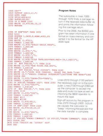
**Fig. 4.** A BASIC-language program to send data from the 9830A calculator's disc drive to a 9-track magnetic tape drive at a remote HP 3000 Computer System.
