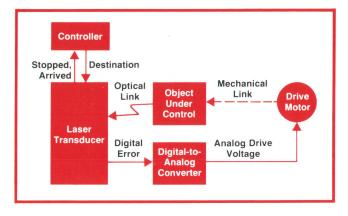
**Fig. 8.** In closed-loop control systems like this one, the laser transducer system receives a destination from the system controller and then takes over the task of moving the object, notifying the controller only when the object stops or arrives at its destination.
