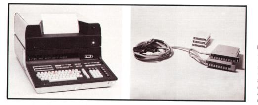
autodialer interface was designed, along with three plug-in data communications ROM blocks (Fig. 1). The Interface Control ROM (Data Comm. 1) must be installed for any data communications application. To convert the calculator to a remote batch terminal, the Binary Synchronous ROM (Data Comm. 2) is also needed. For timesharing applications, the Interactive ROM (Data Comm. 3) is used along with the Interface Control ROM.
