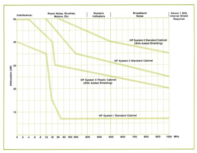
**Fig. 4.** Attenuation of RF energy achieved by the new enclosure design. The values represented are conservative, actual measurements made with a bare enclosure being 10-15 dB greater. The performance actually achieved by any given instrument, however, depends on such matters as the shape and size of holes cut into the panels, on whether metal or plastic control shafts are used, and on the signals present on open connectors.
