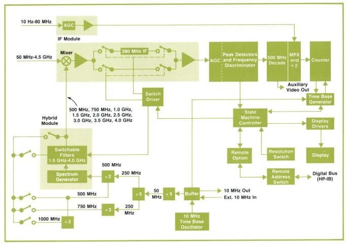
**Fig. 3.** 50-MHz-to-4.5-GHz frequency range is divided into ten bands by switching different local oscillator frequencies to the input mixer. Band switching can be manual or automatic. Two peak detectors and a frequency discriminator control the automatic acquisition algorithm; they also provide diagnostic information.
