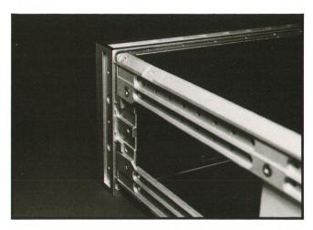
**Fig. 3.** Rear view of the front-panel frame shows the RFI-trap channels into which the top, side and bottom covers are inserted. Ridges provide high-pressure contact points for limiting the wavelength of RF energy that may leak out.
