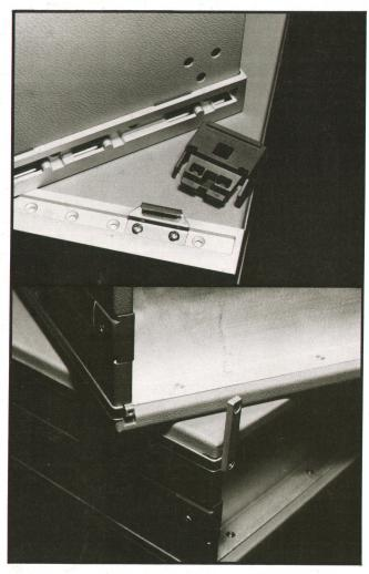
**Fig. 10.** Temporary groupings of instruments are enabled by quick-disconnect links that are fitted to the lower instrument and insert into slots in the front-panel frame of the upper instrument. The rear is retained by straps that bolt to builtin pads. The links also work with horizontal groupings.
