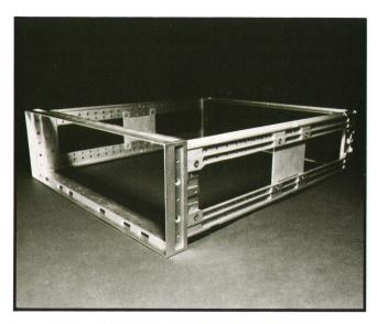
**Fig. 2.** Frame of the new enclosure system. Countersunk holes are for mounting internal parts that have captive nuts. Threaded holes are for attachment of external parts, such as handles, rack-mount brackets, and other fasteners. Slots along the bottom inner edge of the front frame are receptacles for latches that retain plug-ins.
