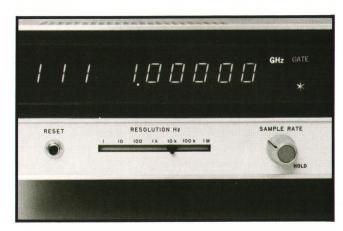
**Fig. 6.** An internal switch causes the counter to display the states of the two peak detectors and the frequency discriminator in the IF channel (three digits at left). These are used with the flow chart of Fig. 7 for troubleshooting.
