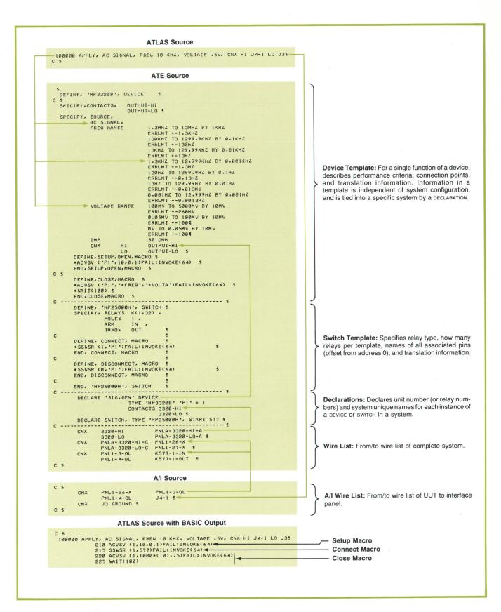
**Fig. 4.** Samples of input code for the ATE and A/l Processors showing relationships with ATLAS source code and the equivalent ATS BASIC output. Arrows at the left show how the ATLAS Compiler compares signal characteristics with device capabilities. Arrows at the right show how the compiler traces signal paths between a device and the unit under test.
