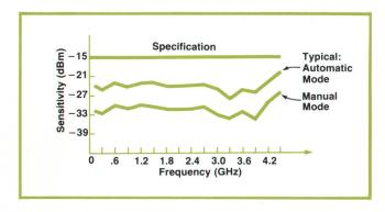
Fig. 2. 5341A sensitivity at  $50\Omega$  input.
