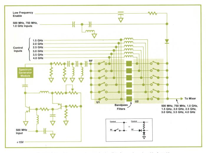
**Fig. 5.** Hybrid module generates the upper local oscillator frequencies and provides for rapid switching from one to another. Worst-case acquisition time for an automatic search of the full frequency range is less than 600 microseconds.
