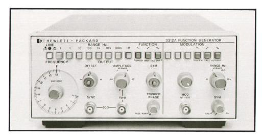
**Fig. 5.** New cabinet design maximizes the available front-panel area for uncrowded control lay-out.
