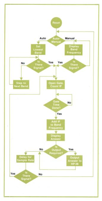
**Fig. 4.** Algorithm for the state machine that controls counter operation.
