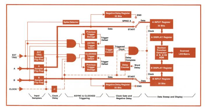
Fig. 9. Logic Analyzer block diagram.
