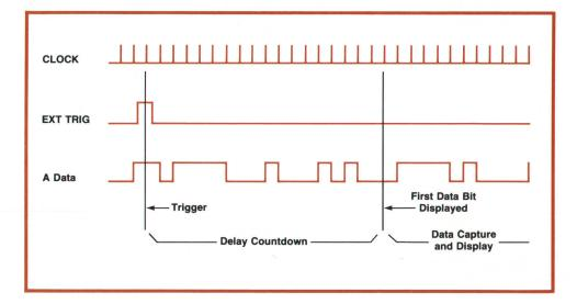
**Fig. 4.** Preset digital delay is counted down between the trigger event and the start of the display. Here the Analyzer triggers when there is a logic HIGH at the EXT TRIG input, and display begins after an 18-clock-pulse delay.
