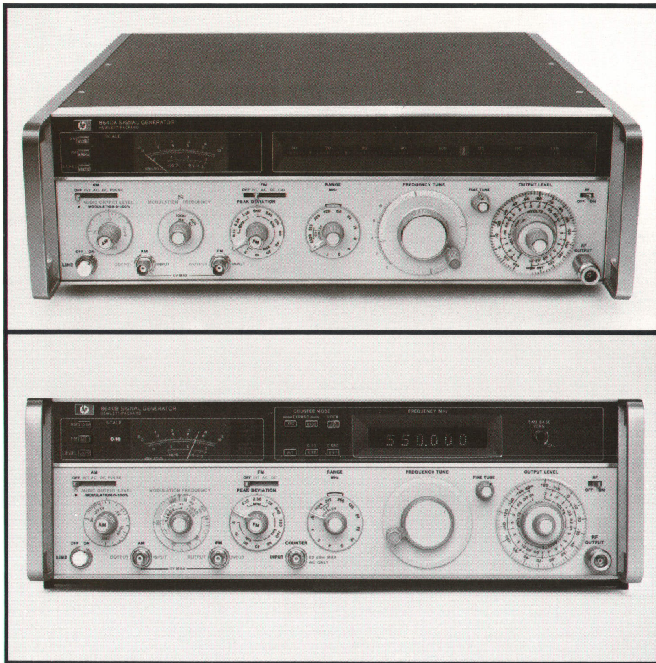
Fig. 1. New Model 8640A solid-state Signal Generator, which covers 450 kHz to 550 MHz range of frequencies, rivals special purpose vacuum-tube generators in spectral purity. Besides highly stable CW signal, new Generator produces modulated signals, both AM and FM, with calibrated modulation. Wide range of output levels, +19 to -145 dBm, meets requirements of broad variety of RF tests.
