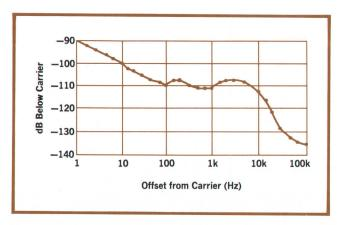
**Fig. 3.** Typical single-sideband phase noise measured at output of Model 3330A/B Automatic Synthesizer in 1-Hz bandwidth with instrument operating at 12 MHz.
