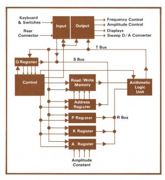
Fig. 7. Principal operation blocks of digital controller.
