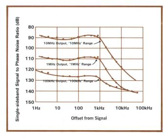
**Fig. 6.** Phase noise of Models 3320A/B Frequency Synthesizers in 1-Hz band referenced to output frequency. Phase noise reduces 20 dB each time instrument is down-ranged until limited by phase noise of 18-MHz 'constant' frequency.
