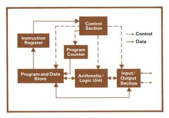
Fig. 2. Generalized block diagram of a digital computer.
