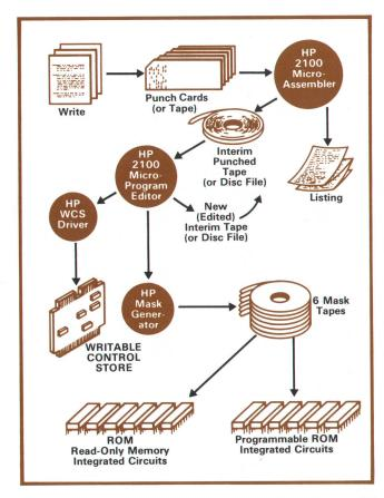
**Fig. 6.** The writable control store package for the HP 2100A Computer includes a microprogramming manual, a microassembler, a WCS editor, a WCS driver, WCS hardware, and a mask generator which produces tapes to be used in manufacturing read-only memories.
