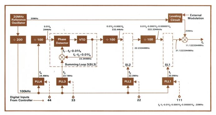
Fig. 4. Simplified block diagram of Automatic Synthesizer frequency generating circuits.
