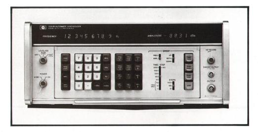
Fig. 1. Model 3330B Automatic Synthesizer is a sweeping frequency standard that allows selection of output frequency with 0.1-Hz resolution in a range of 0.1 Hz to 13 000 999.9 Hz. It also has ac calibrator amplitude accuracy. Built-in digital processor simplifies instrument operation, both by front-panel control or by external programmer.
