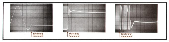
Fig. 5(a). Photo above shows small transient as Synthesizer switches from 10.000 99 MHz to 10.000 00 MHz, a full-range transition for PLL3 (10 MHz has been subtracted from Synthesizer output to clarify presentation).
