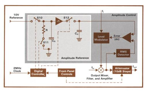
Fig. 8. Elements of Model 3320B amplitude control circuit. RMS detector (thermopile) senses output signal level ahead of step attenuator and produces proportional dc that is compared to reference dc. Any difference (error) modulates level of 20-MHz reference frequency f, to bring mixer output to desired level. Reference dc establishes 1, 0.1, and 0.01 dB digits in output amplitude level. Step attenuator selects 10-dB digits.
