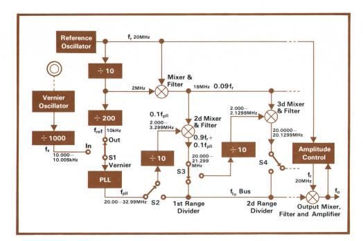
Fig. 5. Simplified block diagram of Models 3320A and 3320B frequency generating circuits shows first two of five divider circuits (seven optional) that reduce span of 'local-oscillator' frequency f₁₀ in decade steps. Switches S2 and S3 are set here to give output range of 0.000−1.299 MHz. To give finer resolution in frequency selection, switch S1 substitutes vernier signal f√ for 10-kHz reference fret.
