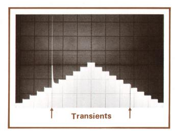
**Fig. 6.** Photo shows 10-step amplitude sweep centered at 3.45 dBm, where 10-dB step attenuator switches and introduces amplitude transients. Amplitude steps are 0.2 dB of 100 ms each. (Oscilloscope sweep speed: 200 ms/cm.)
