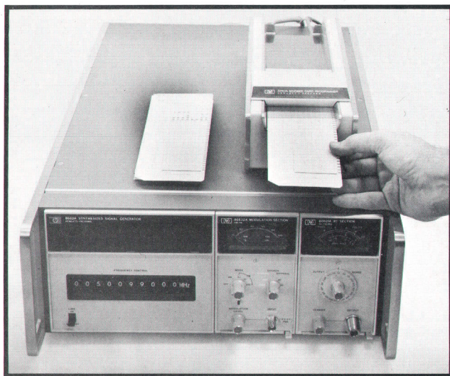
Fig. 11. Synthesizer can be programmed with Model 3260A Marked Card reader.
