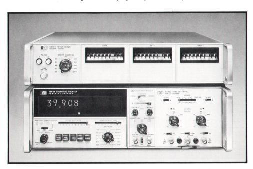
**Fig. 3.** Hewlett-Packard 5360A Computing Counter System makes frequency-stability measurements in either the time domain or the frequency domain. Shown here is the 5360A Computing Counter (lower unit) with the 320 MHz 5365A Input Module, the 5379A Time Interval Plug-in, and the 5376A Programmer (upper unit). In lieu of the 5376A, the 5375A Keyboard may be used as a programming device.
