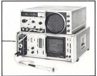
Fig. 5. Complete impedance measuring system includes Probe, Network Analyzer with either or both display plugins, and RF Generator/Sweeper.
