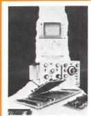
**Cover:** Simplicity of design and operation is implied by HP Journal Art Director Arvid Danielson's photo of parts of the new Model 1810A Sampling Oscilloscope plug-in. Designed for those who would rather not hold the instruction manual in one hand while twiddling knobs with the other, the new Sampling Scope is as
