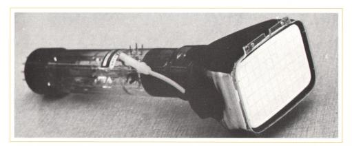
**Fig. 5.** New CRT, only 15 inches long, uses mesh electrode at exit of electron gun to create high-strength electrostatic lens that achieves 3-to-1 deflection magnification in 20 kV post-accelerator field. In addition to reducing power consumption of deflection drive circuits, new CRT uses 1-watt heater for additional power economy.
