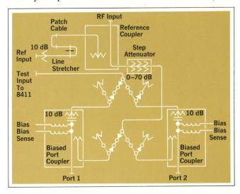
**Fig. 3.** 8746B RF schematic, showing component arrangement and location of the bias circuits. Switches are shown in the  $S_{11}$  position.
