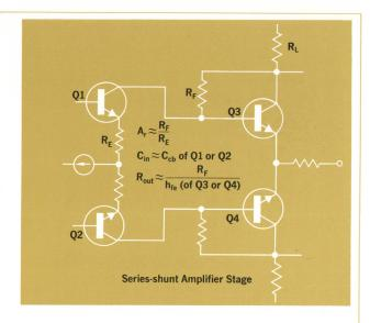
from collector to base in Q3-Q4). The low input capacitance and low output resistance of this type of amplifier means wideband performance at relatively low current. Two of these stages have enough gain to build up the signal sufficiently for driving the output stage.
