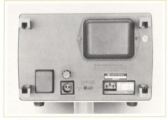
**Fig. 3.** Power mode switch on instrument rear panel selects source of power: ac line, dc line, optional internal battery. AC line input module conforms to new IEC international recommendations for power-line inputs. Module, winner of a 1970 WESCON industrial design award, makes certain that change from 115 to 230 V operation cannot be made unless ac line fuse is removed, making it unlikely that proper fuse change is overlooked.
