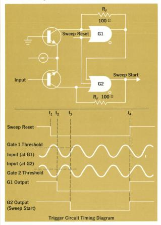
Reset is effected through a second gate. As shown in the diagram, the output of G1 is fed to G2, so anytime that G1 goes high, G2 is forced into the high state.
