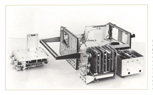
Fig. 7. Vertical amplifier, horizontal amplifier, and power supply are in separate modules that can be tested individually before final assembly. This, plus reduction in internal adjustments, reduces costs by shortening final test and alignment time. Sweep circuits and power supply have removable plug-in boards that can be changed in field to speed service turnaround time.
