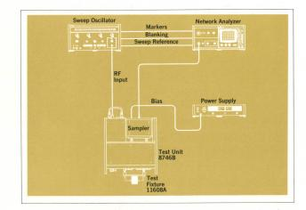
Fig. 2. The HP 8410 Network Analyzer measurement system with the 8746B and 11608A connected into the system.
