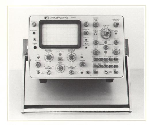
Fig. 2. Despite versatility of new Oscilloscopes (dual-trace display, delayed sweep, triggered sweeps), careful layout of controls make these instruments easy to operate. Black band around push-buttons disappears when a button is pressed, clearly showing that button is in depressed position.
