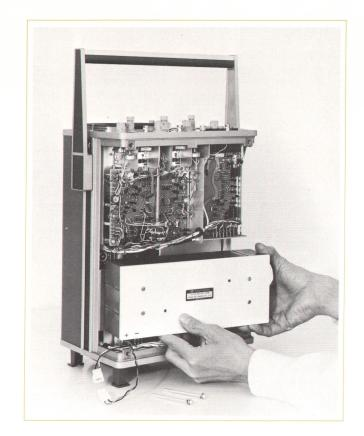
**Fig. 4.** Optional battery pack mounts entirely within oscilloscope with only two screws and one connector. No modification of scope's circuits are required—battery can be added or removed at any time.
