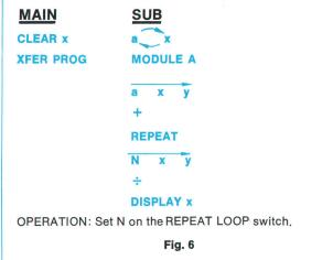
ber of samples included in a calculation. The current setting of the REPEAT LOOP switch can be read into the x register using the 34 instruction, and can be used in the calculations. An example of a looping program for finding a simple average is shown in Fig. 6.
