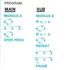
OPERATION: Set N on the REPEAT LOOPswitch. Set PAUSE DISPLAY = ON. If PAUSE HALT is OFF, program will run continuously, displaying Range = Max - Min. If PAUSE HALT is ON, program will stop after each display; the maximum measurement can be read out with  $\overline{a \times y}$ , and the minimum with  $\overline{b \times y}$ .
