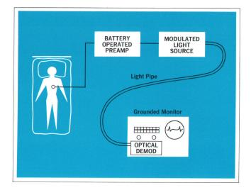
Fig. 6. Excellent isolation can be provided by optical coupling but technique is not economically feasible at present.
