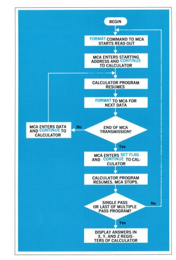
Fig. 3. Simplified flow chart of multichannel-analyzer/ calculator operation.
