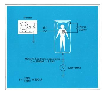
**Fig. 3.** Equivalent circuit of situation diagrammed in Fig. 2.
