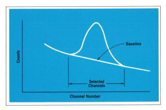
**Fig. 5.** Typical of the tasks the calculator can do is fitting a baseline to a peak, then subtracting the baseline to leave only the significant data.
