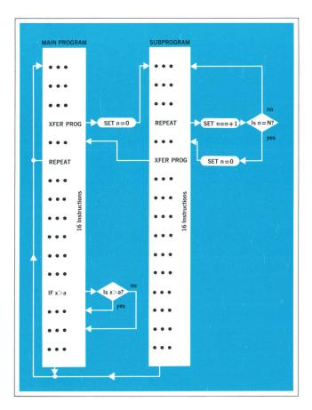
**Fig. 2.** Model 5375A Keyboard has two memories of sixteen program steps each. The XFER PROG key transfers control from one to the other. The IF keys are for program branching and the REPEAT key is for looping.
