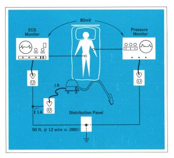
**Fig. 4.** If all equipment near patient is not connected directly to common ground point, a hazardous situation can develop. Leakage current in vacuum cleaner here is sufficient to create voltage dangerous to patient.
