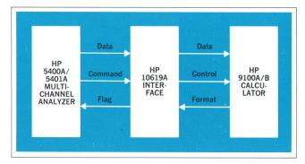
**Fig. 2.** Two interface cards plugged into the multichannel analyzer allow it to communicate with the HP calculator. The calculator is programmable, easy to use, and fast, and it can reduce most analyzer data just as well as a computer.
