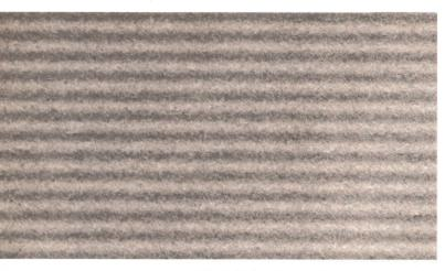
Fig. 4. Unity interlace factor means spacing between adjacent raster lines is constant.
