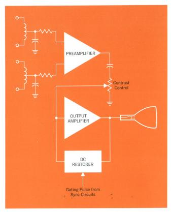
Fig. 2. Picture amplifier has loop-through balanced or unbalanced inputs for standard television and telephone cables. Do restorer maintains luminance of displayed black signals constant within 1%. Frequency and phase responses are carefully controlled to avoid distortion.
