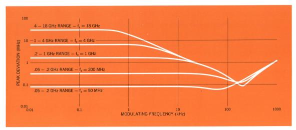
Fig. 4. Phase-lock loop remains locked to FM signals having peak frequency deviations and modulation frequencies indicated. For example, if input signal has carrier frequency  $f_{\kappa}=18$  GHz, loop will remain locked for sinusoidal FM of frequency 20 kHz and peak deviation 1 MHz. If modulating frequency is only 300 Hz, peak deviation can be 30 MHz.
