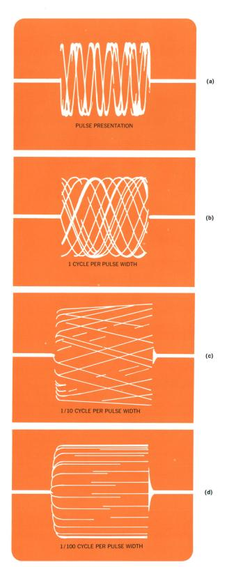
Fig. 6. Typical waveforms at sampler output while tuning for zero beat (oscilloscope not synchronized to RF carrier). Stability of VFO of new transfer oscillator is high enough to permit tuning within 1/100 cycle per pulse width of zero beat, i.e. within (100 × pulse width)<sup>-1</sup> Hz. See Fig. 7.
