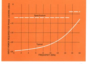
Fig. 1. The new HP Model 5257A Transfer Oscillator, a plug-in for several HP electronic counters, phase-locks reliably to input signals as small as -24 dBm at 50 MHz and -8 dBm at 18 GHz.
