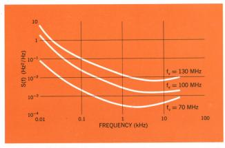
Fig. 8. Frequency spectral density of VFO of Model 5257A Transfer Oscillator. Short-term rms frequency fluctuations are only about 1 part in 107.
