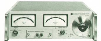
Fig. 1. This low-frequency -hp- Model 4800A Vector Impedance Meter makes rapid measurements of components and circuits with direct readout over the frequency range from 5 Hz to 500 kHz, and over the impedance range from 10 ohms full scale to 10 megohms full scale.
