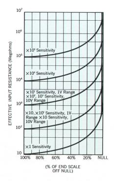
Fig. 3. Input resistance to the -hp- Model 3420A/B approaches infinity as the null is approached. Input resistance at the null is determined only by leakage resistance of switches and wiring.
