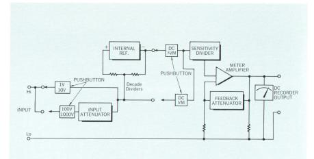
Fig. 2. In the differential voltmeter mode, the floating voltagereference supply is used to drive the precision decade dividers. On the 1-volt and 10-volt ranges the input voltage is nulled directly against the 6-digit dividers. On the 100-volt and 1K-volt ranges the input voltage is divided to the 1-volt level and then nulled with the decades. The instrument can also be used as a dc voltmeter with the reference disconnected.
