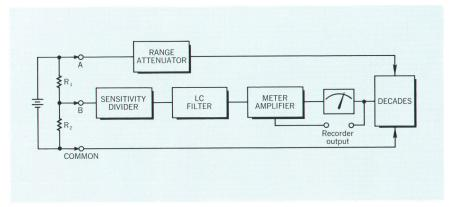
Fig. 4. In the ratiometer mode of operation, the -hp-Model 3420A/B acts as a modified Wheatstone bridge to make voltage and resistance divider measurements. The range attenuator and decade divider make up one side of the bridge and the meter amplifier acts as the null detector. The connections from A to COMMON null detector. Connections from A to COMMON and B to COMMON are the other side of the bridge.
