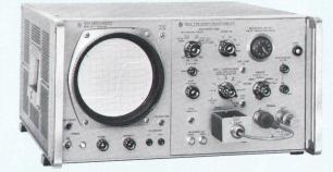
Fig. 2. Rise time converter is placed between STEP OUTPUT and SIGNAL IN connectors of -hp- TDR system, which consists of Model 1415A TDR Plug-in for Model 140A Oscilloscope.
