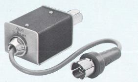
Fig. 1. New rise time converters, -hp- Models 10452A to 10456A, slow the rise time of the voltage step in the -hp- TDR system to 0.5, 1.0, 2.0, 5.0, or 10.0 nanoseconds to simplify testing of band-limited systems. Rise time of -hp- system without converters is 0.15 ns. Shown is 5 ns converter, Model 10455A.
