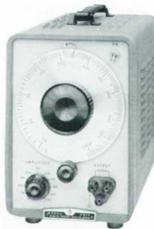
Fig. 2. (right) New -hp- Model 207A oscillator covers complete 20 cps-20 kc range in single band, has shaft extension at rear to enable it to be used with external motor drives for automatic audio response measurements on amplifiers, transformers, speakers, and other audio devices. No zero setting is required. Log dial facilitates response plots on scope or recorder.
