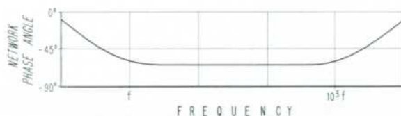
Fig. 6. Phase characteristic of synthesized network. Deviation over rated range is less than a few degrees.
