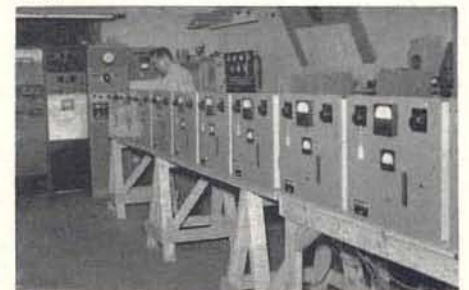
George Hanawalt is making daily check during two week tests on MO-2639 Frequency Monitor.
