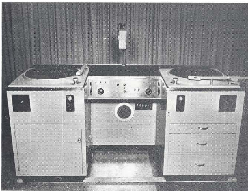
Radio Station KXYZ's technical Supervisor Gerald R. Chinski has forwarded to us this picture of the custom built announcer's transcription console and work desk which was built using Gates CB7 Turntable and Gates MO 2716 Reproducer Assembly. Fine job, boys.
