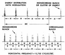
Fig. 13—Interleaving of brightness signal and chroma signal using sideband spacing effect.
