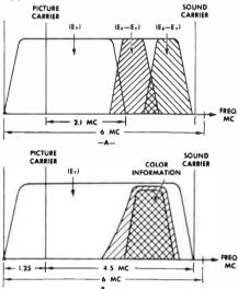
Fig. 11—Two methods of sharing 6 mc band. This would mean that some portion of the 6 megacycle band must be shared by both the high definition brightness signal and the low definition color information. The next step is to determine how this could be accomplished.
