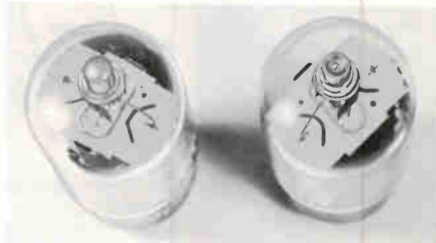
Fig. 1. Top view of soldered top cap, left, and the new General Electric welded top cap, right.
