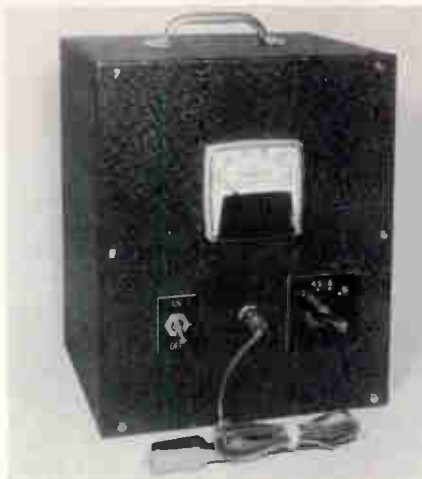
Fig. 1 Completely assembled power supply for servicing transistor radios.
