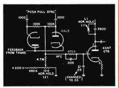
Changed  $C_1$  from .05 to .03 (changing time constant) and readjusted  $L_1$ . This corrected sync problem and set has operated satisfactorily ever since.
