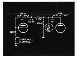
This is a very common complaint on these and similar models. Solution usually lies in replacement of C2, .001 mfd capacitor. This capaitor may be either leaky or completely shorted. High incidence of failure is caused by high pulse voltages present. Replacement should be a high quality unit rated at 600V or higher.
