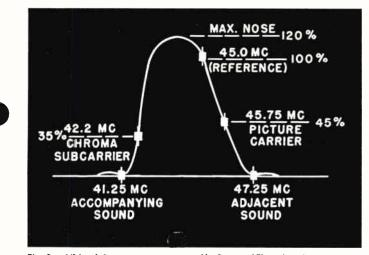
Fig. 2. Video i-f response curve used in General Electric color receiver.
