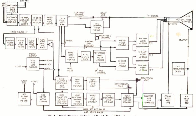
Fig. 1. Block diagram of General Electric Type "CL" color receiver.
