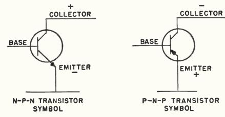
Fig. 2. N-P-N and P-N-P transistor symbols.
