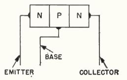
Fig. 3. Arrangement of elements in junction type transistors.
