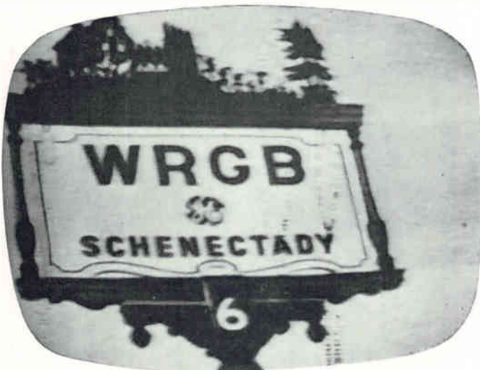
TELE-CLUE E-207 —This shows the effect of "snivets" when a picture is received. A different horizontal output tube may eliminate the "snivets" entirely or change the frequency so the picture is "clean." Another method which may be used is to place an ion-trap magnet over the horizontal output tube as shown in the photographs on the right. The ion-trap is then slowly turned until the "snivets" disappear.
