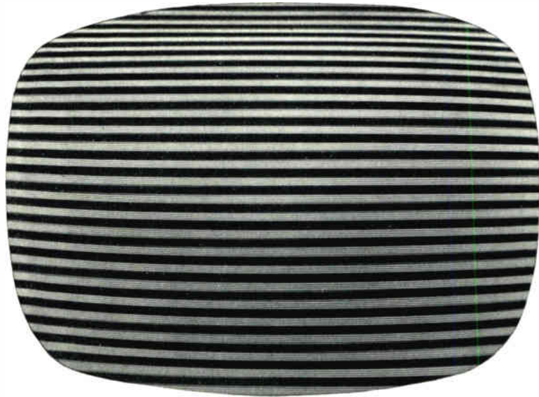
Figure 5. 1500-cycle modulation with poor vertical linearity.
