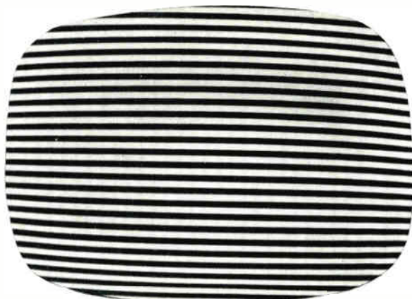
Figure 3. Pattern produced by signal generator with 1500-cycle modulation.
