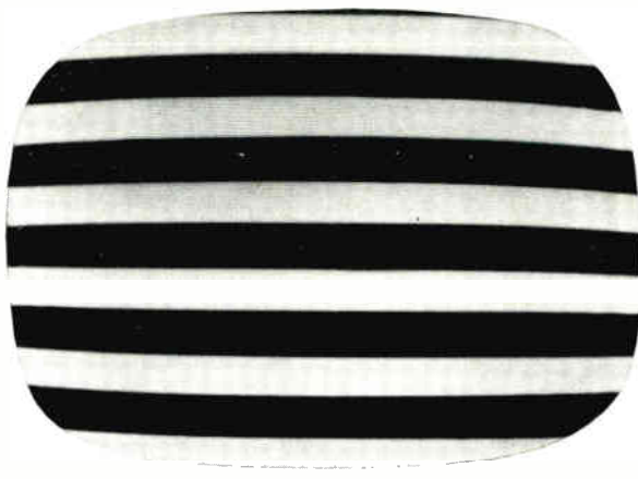
Figure 1. Pattern produced by signal generator with 400-cycle modulation.
