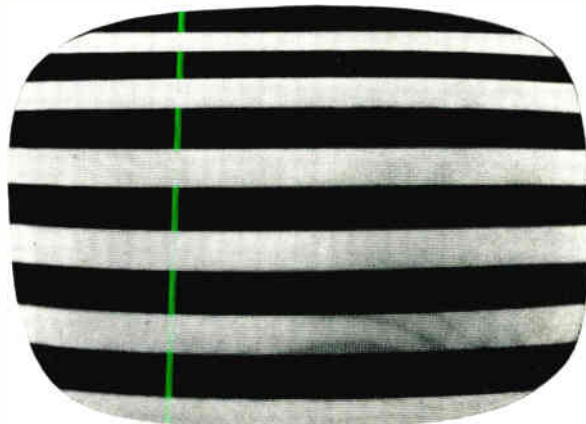
Figure 4. 400-cycle modulation with poor vertical linearity
