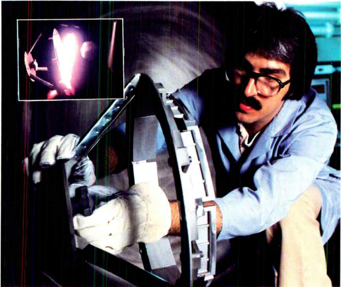
A technician at Aircraft Engine Business Group prepares the vacuum chamber for plasma spraying (inset).
