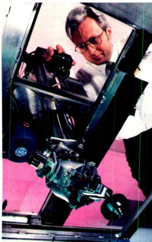
R&D engineer Allen W. Case, Jr., installs GE solid-state TV camera on an experimental assembler.
