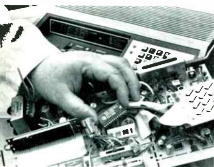
New GE AM/FM programmable digital clock radio uses microcircuits to provide such new features as different wake-up times, different stations for slumber and wake-up, and a memory to allow recall of six pre-selected stations (see page 26).
