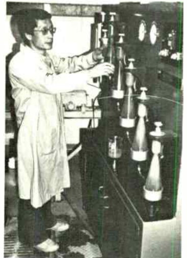
To produce tungsten concentrates, various chemical reagents and flotation processes must be tested. Below, technician Emilio Cruz sets up a pilot plant leaching apparatus.
