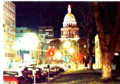
A city street in Denver, Colo., is lit with 400-watt Lucalox® lamps, which give six to eight times more light than the lamps they replaced.
