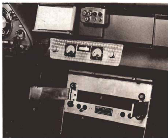
W8WFH (front) and W8DLD run power output tests on the completed LWM-3 SSB/CW transceiver, running it into a 50-ohm dummy antenna load. Vacuum-tube voltmeter is measuring RF voltage across load, providing power output indication.
