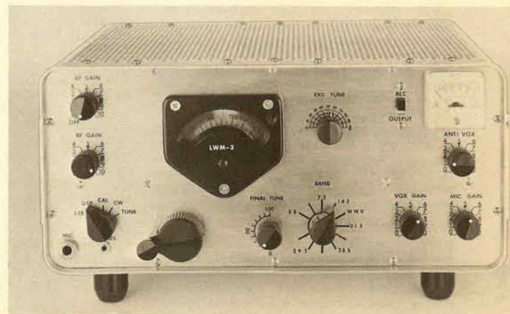
FRONT-PANEL VIEW of the beautifully constructed LWM-3 transceiver. All controls used during normal operation are at the left, easily accessible from the driver's seat. This model has been seen by thousands of radio amateurs at meetings and conventions during 1961. Panel has brushed aluminum finish.
