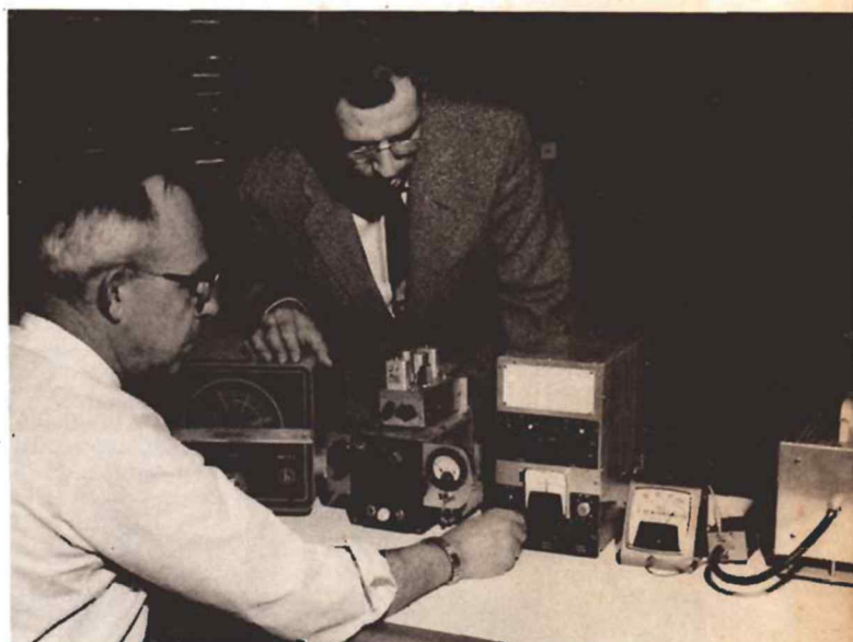
W8DLD (left) and W8WFH put their RF wattmeter through its paces, checking it against the RF wattmeter built into the SSB-600 linear amplifier (center unit). Converted Command set receiver and crystal controlled converter at left of SSB-600 was described in the September-October, 1960 issue of G-E HAM NEWS .
