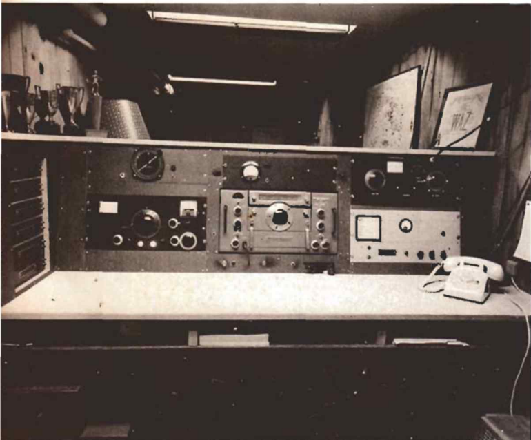
MODERN HETRODYNE EXCITER in W2FBS's attractive station console has the two-tube differential keyer unit built right into it. Exciter will be described in the July-August, 1961 issue. In addition to four one-kilowatt power amplifiers for the DX bands, the station also has a PI-NETWORK ANTENNA TUNER at right (see G-E HAM NEWS , May-June, 1960, page 3). World map in background contains 260-odd pins representing the present DXCC score on CW at W2FBS.
