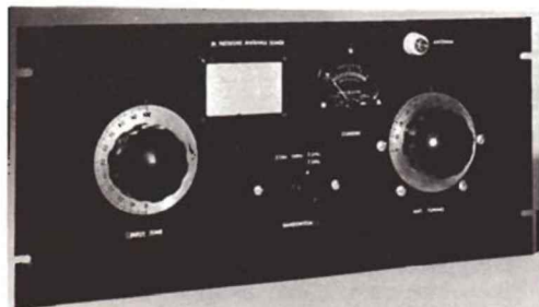
PANEL VIEW of the one-kilowatt pi-network antenna tuner at W2FBS, constructed on an 8 3/4 x 19-inch aluminum relay rack panel. National type "0" dials are on C 1 and C 2 .
