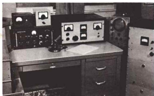
MONITOR-ADAPTED 'SCOPE AT K21OW, at right of desk, a Heath type O-5 constructed from a kit. Space for the adapter components and additional panel controls can be found in most test type oscilloscopes.
