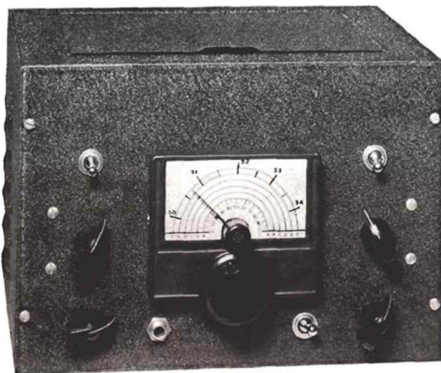
Fig. 1. Front panel view of six-meter receiver. Controls in bottom row, left to right, are audio gain, headphone jack, AVC switch and r-f gain. The BFO control and switch are at upper left, and ANL control and switch at upper right.
