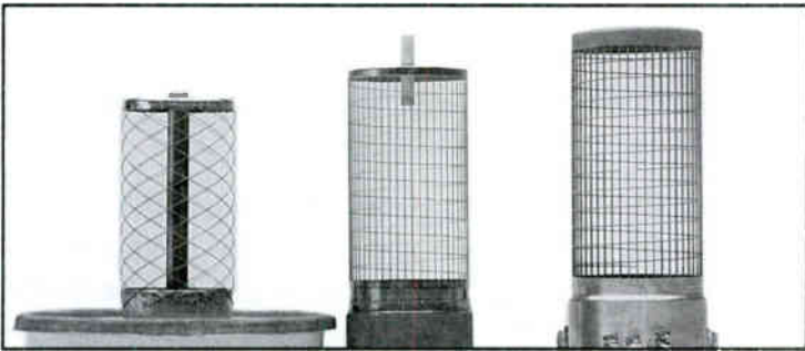
Interior elements of a tetrode. Mesh filament on the left, control grid center and screen grid on right
