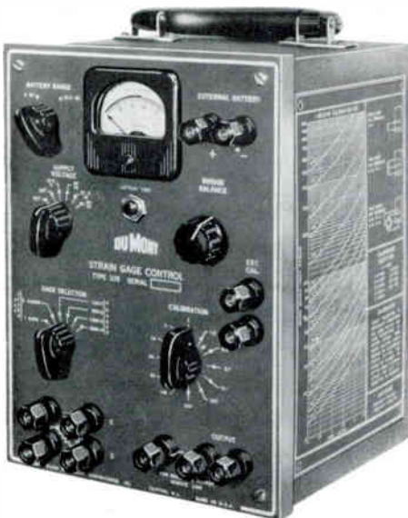
Fig. 1. The Du Mont Type 335 Strain Gage Control. A self-powered instrument containing the control and calibrating circuitry for resistance-type strain gages. Gage factors from 1.5 to 4 can be handled easily and conveniently.
