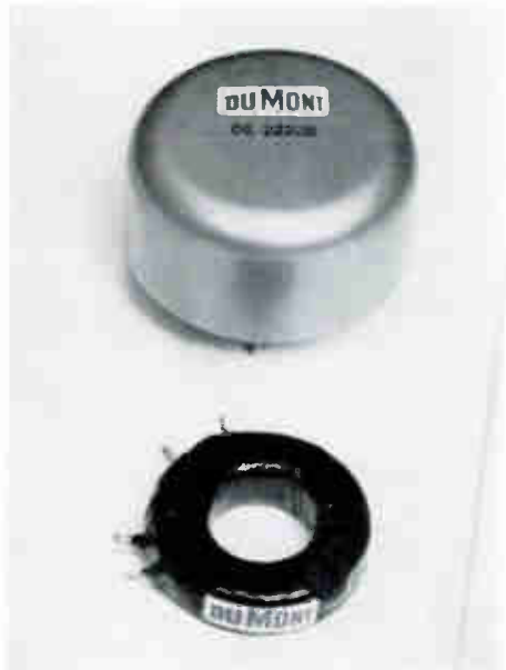
Newest type Du Mont Pulse Transformers. Miniaturization of components such as these have made possible smaller and more accurate systems for varied applications.
