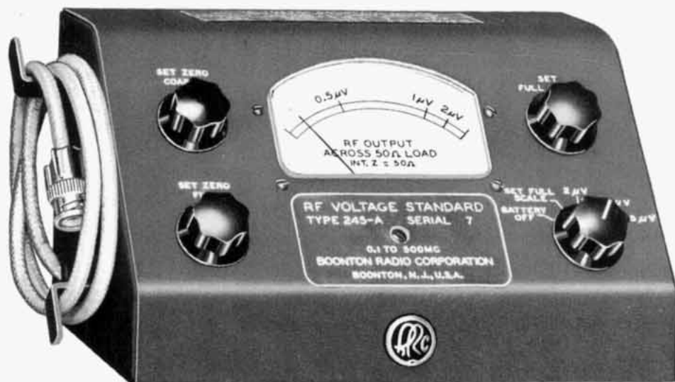
Figure 1. The RF Voltage Standard Type 245-A.
