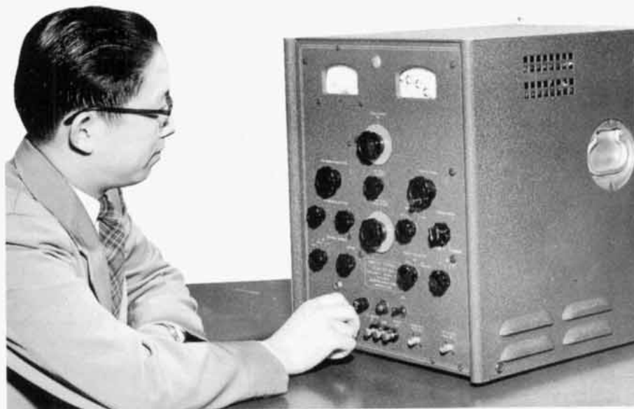
Figure 1. Dr. C. L. Kang, co-author, adjusts the Sweep Signal Generator Type 240-A.
