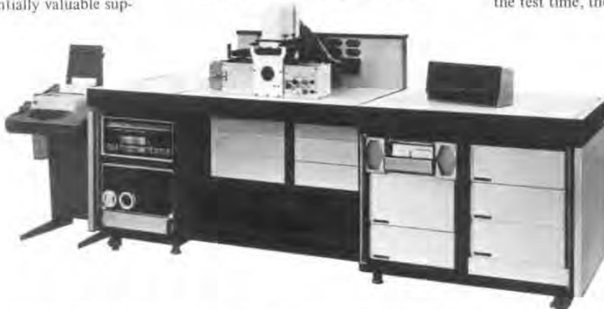
GR's Type 2240 Resistance Anodize Trim System trims 144 resistors at a time on a thin-film tantalum substrate.
