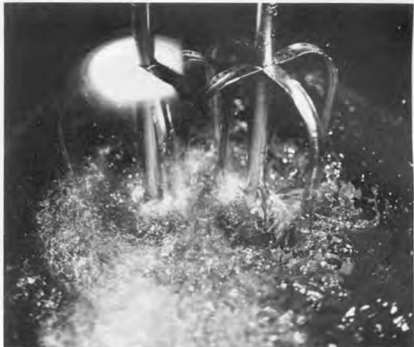
An unretouched photograph showing one beater blade whirling under normal lighting conditions while the second blade is visually stopped by stroboscopic light, although the liquid continues to churn beneath it!
