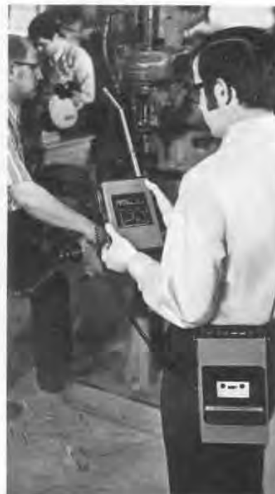
The 1933 indicates the current noise level in a machine shop, while the 1935 continuously records the changing level for exposure analysis according to OSHA requirements.
