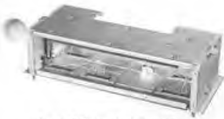
A typical device adaptor used in network-testing systems.
