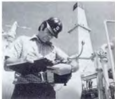
With soundproofed oil-drilling derrick towering behind him, Standard engineer uses GR octave-band noise analyzer to check effectiveness of noise-reduction measures at drill site.
