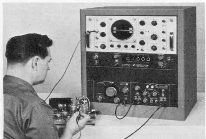
Figure 15. Rack-mounted Type 1310-A Oscillator and Type 1396-A Tone-Burst Generator used to test amplifier overload characteristics. A behind-the-panel connection to the synchronization jack allows precise readout of frequency on the Type 1150-B Digital Frequency Meter.
