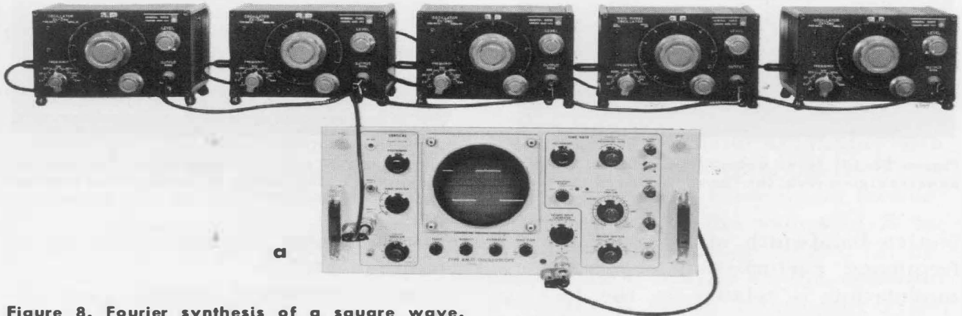
Figure 8. Fourier synthesis of a square wave. (a) Five oscillators synchronized to the first five odd-order harmonics of a square wave. The sinusoidal outputs of the oscillators are adjusted for phase coherence and summed in the ratio of their respective Fourier coefficients to make a Fourier approximation to the original square wave. (b) The original synchronizing square wave. (c) The coherent fifth harmonic. (d) The synthesized square wave.
