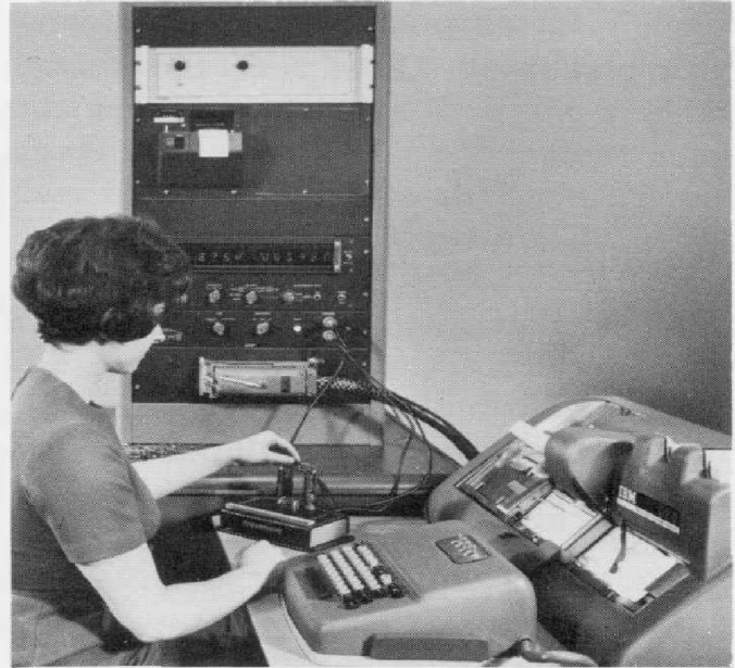
Fig. 9. IBM Model Printing Summary Punch operating from output of automatic bridge. Capacitance values are automatically punched; operator adds serial numbers. Also in relay rack are data printer and (top) intercoupler required for parallel-to-serial conversion.
