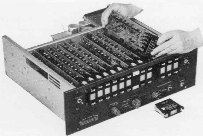
Figure 10. Plug-in etched boards are easily removed for service or replacement.
